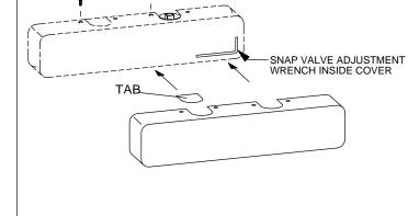
Place tab in cover slot opposite main arm. Place cover over closer and fasten securely with
