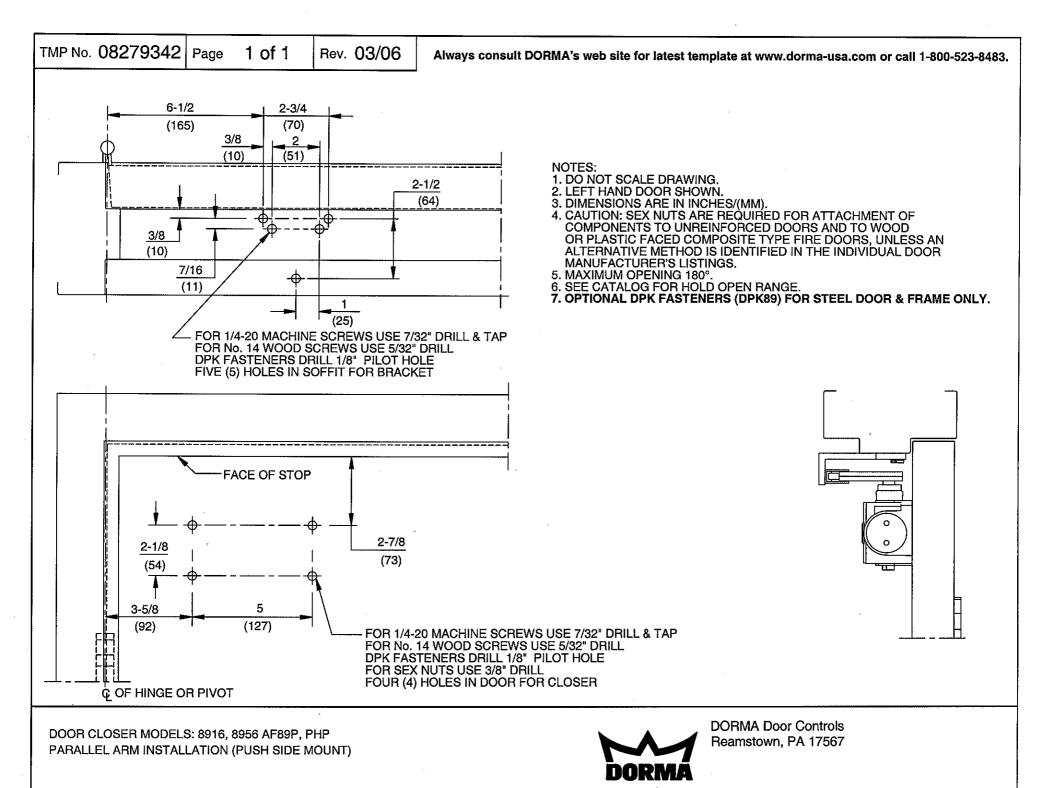
DOOR CLOSER MODELS: 8916, 8956 AF89P, PHP PARALLEL ARM INSTALLATION (PUSH SIDE MOUNT) WITH PLATE DP89
