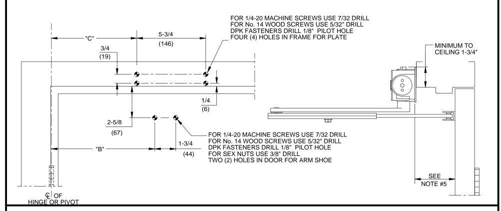
DOOR CLOSER MODELS: CLSC16HD TOP JAMB DROP INSTALLATION (PUSH SIDE MOUNT) WITH PLATE BP89
