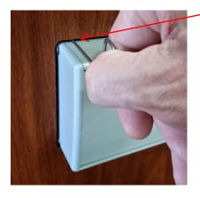
Move the tool inward following the end cap. Once the tool clears the bottom of the end cap, move the tool sideways (approx. 3/8") away from where the tool was inserted. The tool will engage the Hold/Release link at this point.
