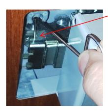
Close up view showing the release tool engaging the release link.
