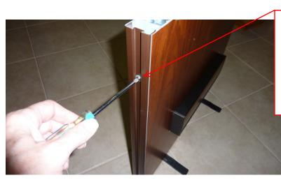
Remove the door edge by loosening all screws along the vertical edge. The screw arrangement varies depending on the door edge configuration.
