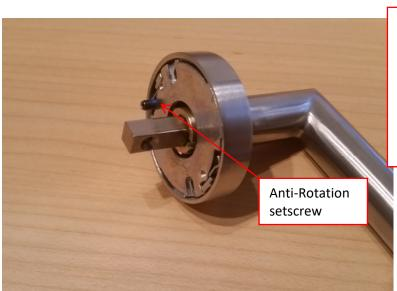
Each handle set is preassembled as shown. The protruding setscrew mates with a corresponding hole in the door face to prevent the rose from rotating once installed.
