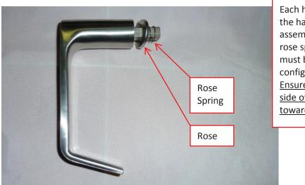
Each handle set includes the handle/shaft assembly, rose, and the rose spring. The handle must be installed configured as shown. Ensure that the recessed side of the rose is facing towards the door.
