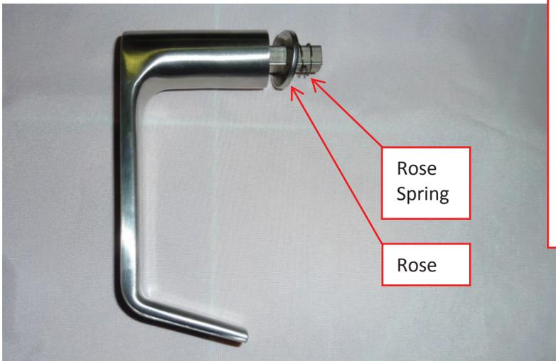
Each handle set includes the handle/shaft assembly, rose, and the rose spring. The handle must be installed configured as shown. Ensure that the recessed side of the rose is facing towards the door.
