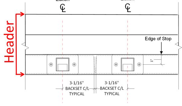
Syntégra uses top latching as a standard for XT, PX, and LX Door Systems.
