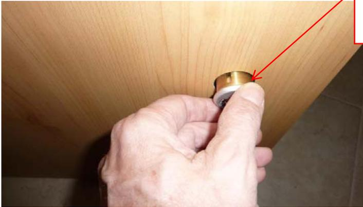
Insert the cylinder into the lock case opening.
