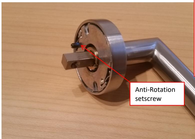
Each handle set is pre-assembled as shown. The protruding setscrew mates with a corresponding hole in the door face to prevent the rose from rotating once installed.
