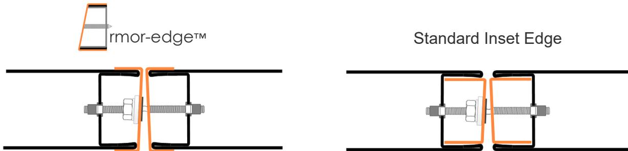
Created to complement the aesthetics of the Syntégra Integrated Door Systems, Armor-edge strikes a distinctive balance between beauty and strength. Armor-edge, used in conjunction with Syntégra's HG Series continuous hinge, frames the door with stainless steel to provide full protection for both edges.
