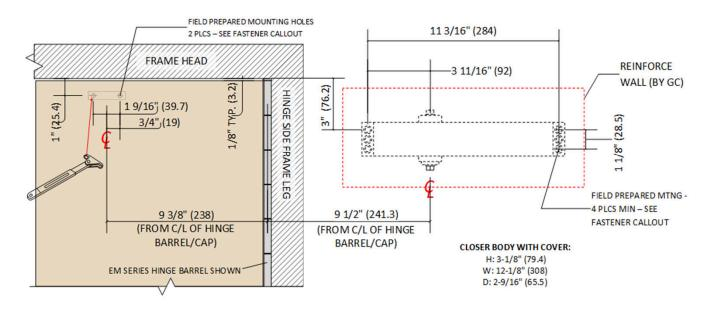
This template supports standard Syntégra EMA/EM Hinges, and 4-½" butt hinges only! Contact factory for other hinge types.
