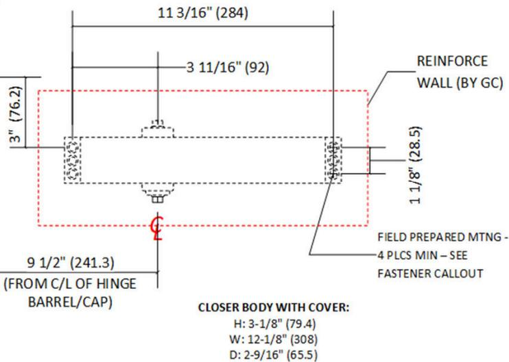
This template supports standard Syntégra EMA/EM Hinges, and **4-½" butt hinges only!** Contact factory for other hinge types.
